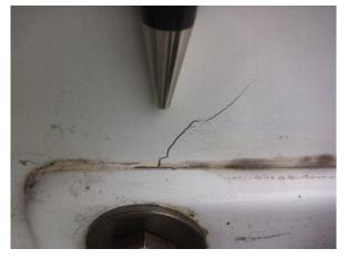
The Lewmar electric windlass, mounted in the anchor locker is bolted to a bulkhead. This bulkhead is deflected forward by up to 4mm and cracks in the gel coat have formed at the top joint and corners.
