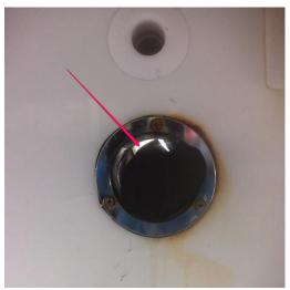
There are two aft cockpit drains located port and starboard in the transom, these have rubber flaps to prevent water coming into the cockpit when motoring astern or in a following sea. Both these flaps are perished and split. It is recommended these flaps are replaced prior to re launching the boat.
