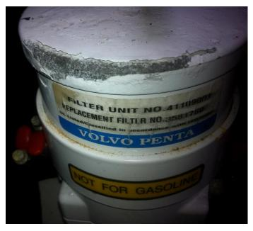
The primary Diesel fuel filter is showing signs of corrosion, whilst this is only a cosmetic issue, you may consider having this taken back to bare metal, an alloy primer and appropriate paint to bring this back to good condition.
